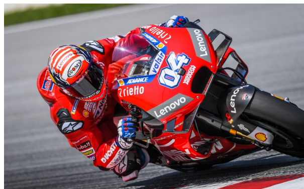
Figure 1.1: Example of a side-wings configuration integrated on the MotoGP fairings for the 2019 season.
